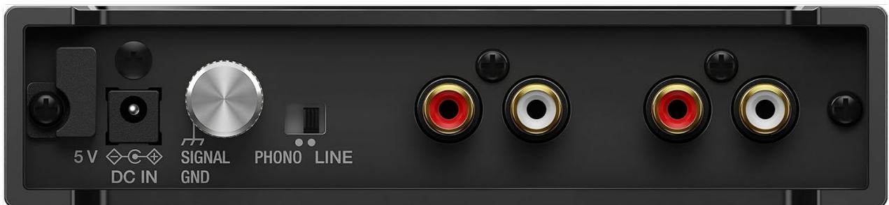
Image: Rear panel of the Pioneer DJ INTERFACE 2, showing the input/output ports, USB, DC IN, and GND terminal. After physical connections, install the rekordbox software and drivers on your computer. Launch rekordbox and configure the audio settings to recognize the INTERFACE 2 for DVS control.
