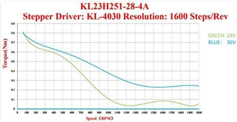
Figure 4: Torque-speed curve for the KL23H251-28-4A stepper motor, showing performance with a KL-4030 driver at 24V (green) and 36V (blue).
