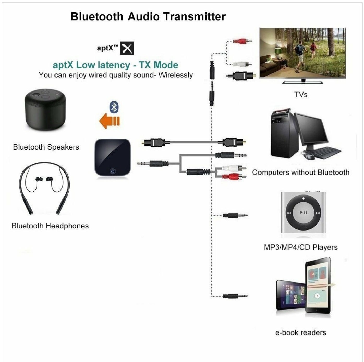
Image 4: Diagram illustrating the Bluetooth Audio Transmitter (TX) mode, showing connections from TV, PC, MP3 players, and e-book readers to Bluetooth speakers and headphones.
