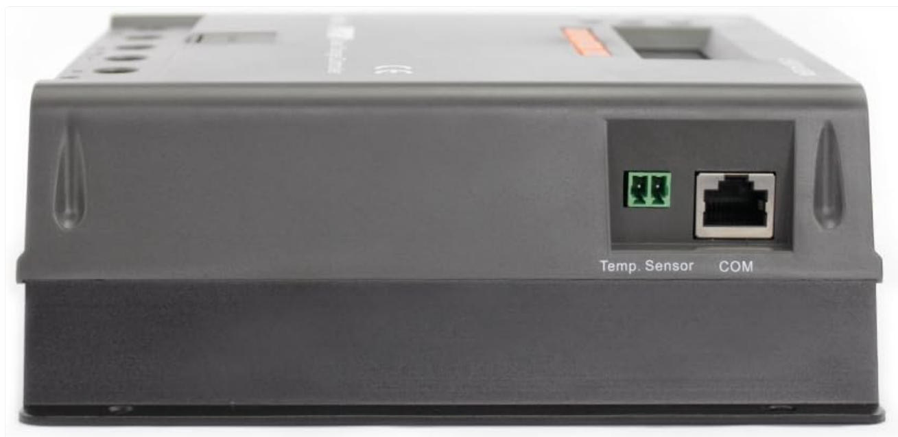
Figure 4.4: Side View with Communication Ports. This image shows one side of the controller, featuring the "Temp. Sensor" port (green terminal block) and the "COM" (RS485) port (RJ45 connector) for external communication and temperature sensing.
