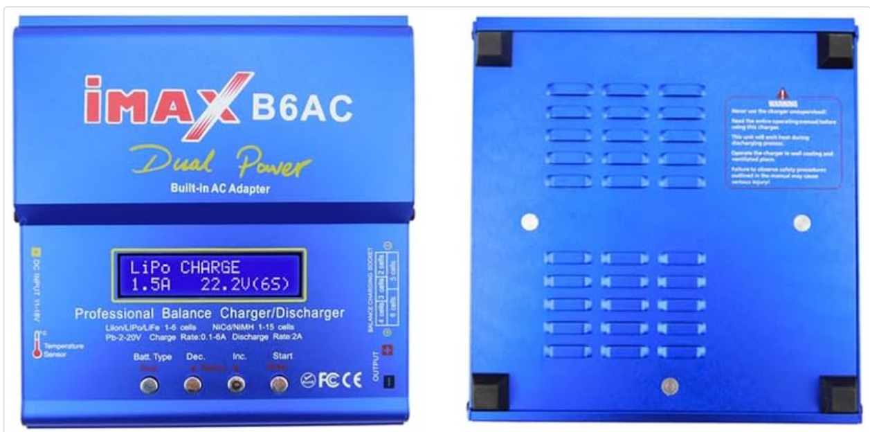
Image 4.2: This image displays both the front panel and the bottom of the IMAX B6AC charger, revealing the ventilation grilles on the bottom for heat dissipation and important warning labels regarding operation and safety.
