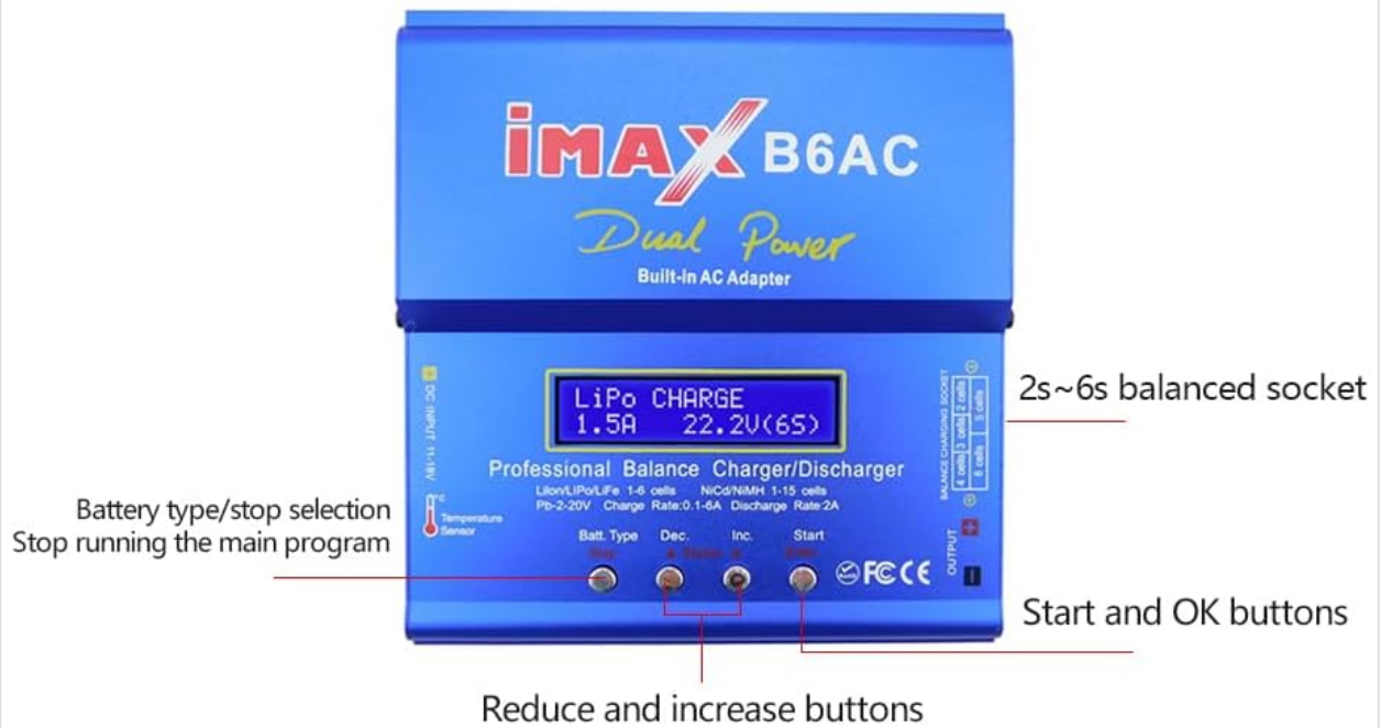
Image 6.1: An annotated image of the IMAX B6AC charger's control panel, clearly labeling the functions of each button: 'Batt. Type/Stop' for selecting battery type and stopping programs, 'Dec' for decreasing values, 'Inc' for increasing values, and 'Start/Enter' for initiating processes and confirming selections.
