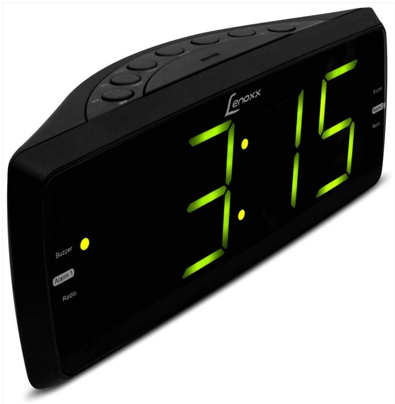
Figure 1: Front view of the Lenoxx RR736 Clock Radio, displaying the time 3:15 in green LED digits. The front panel also shows indicators for Alarm 1 (Buzzer/Radio) and Alarm 2 (Buzzer/Radio).
