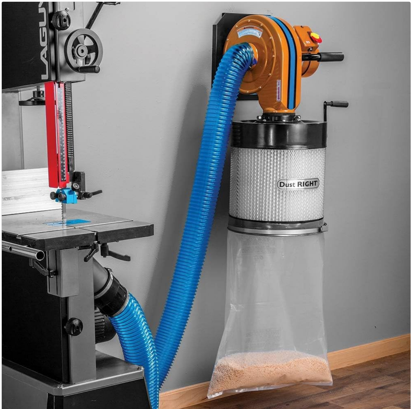
Image: The Dust Right Canister Filter shown installed beneath a wall-mounted dust collector unit, connected by a blue flexible hose to a
