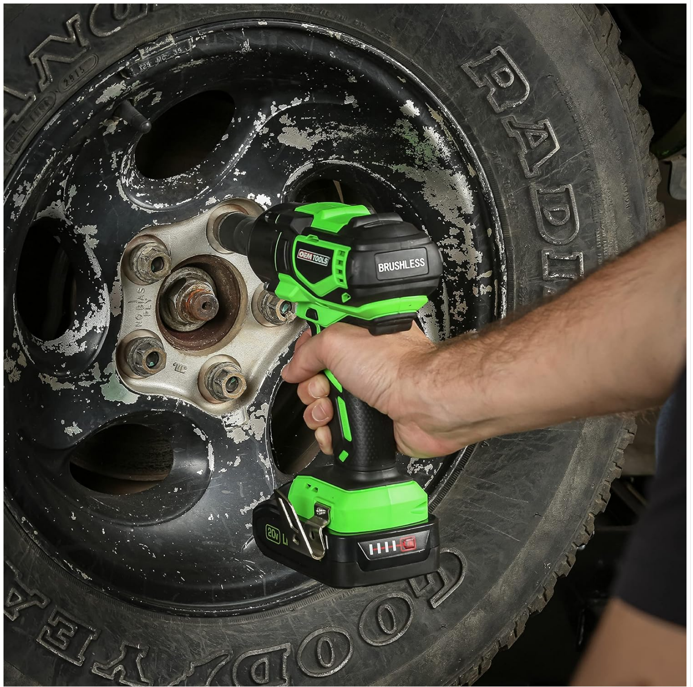
Figure 6: The impact wrench in use, removing a lug nut from a vehicle tire.
