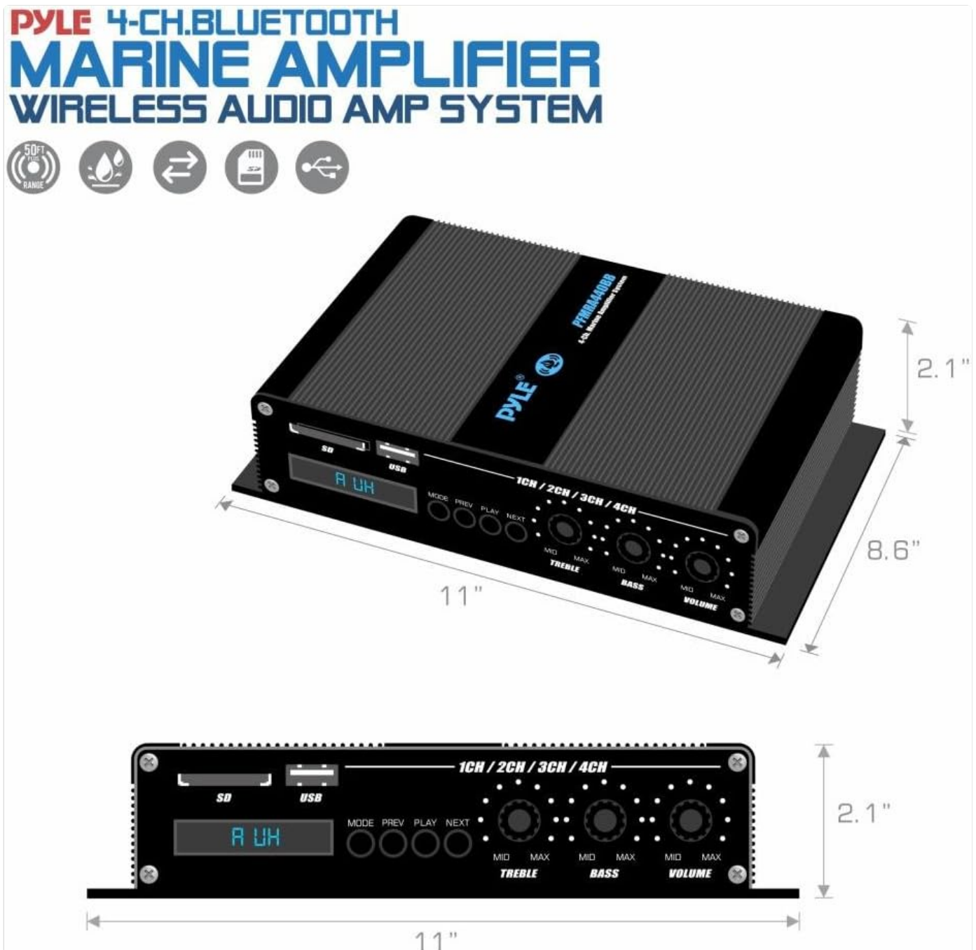
Figure 4: Dimensional drawing of the PFMRA440BB amplifier.
