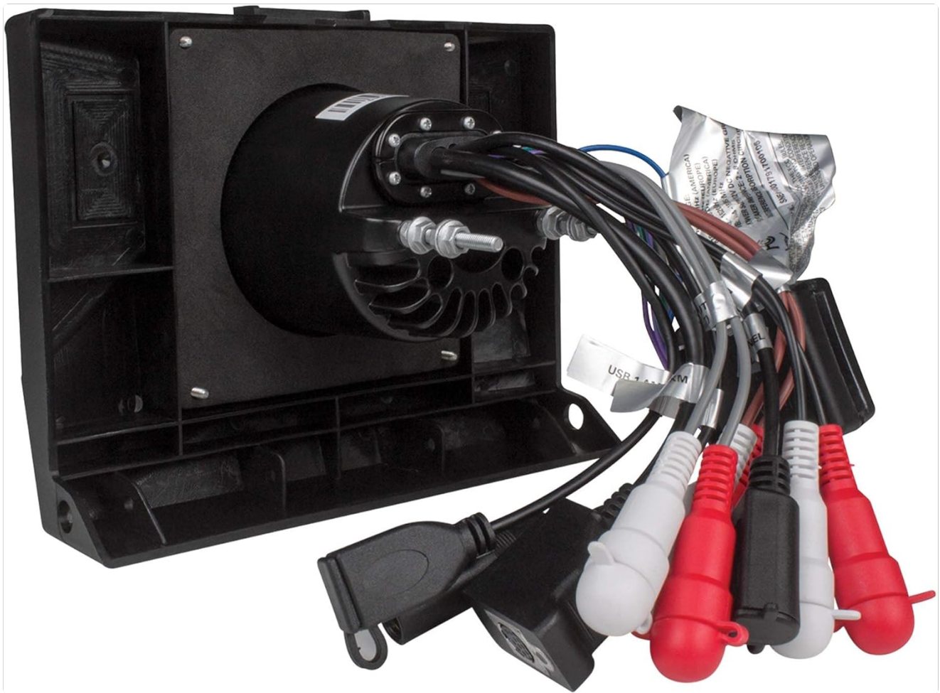
Figure 6: Close-up of various connections including USB, RCA pre-outs, and the main power/speaker harness.
