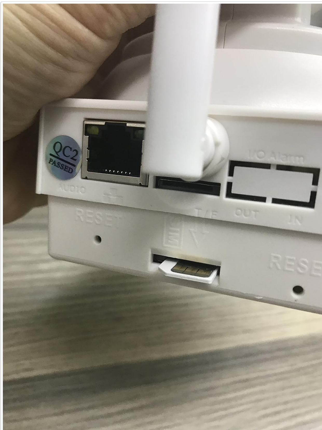
Figure 4.3: Detailed view of the SIM card slot and MicroSD card slot, located on the underside or side of the camera base.
