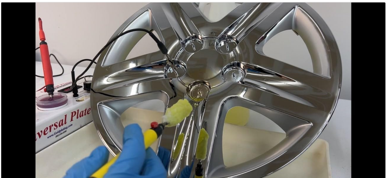
Initial setup of the Universal Plater, showing the console, solutions, and a chrome wheel ready for processing. An applicator wand is connected and in use.
