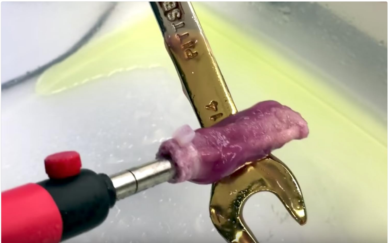
A close-up view of a wrench undergoing the chrome stripping process. The applicator wand is applying a purple solution to remove the chrome layer.
