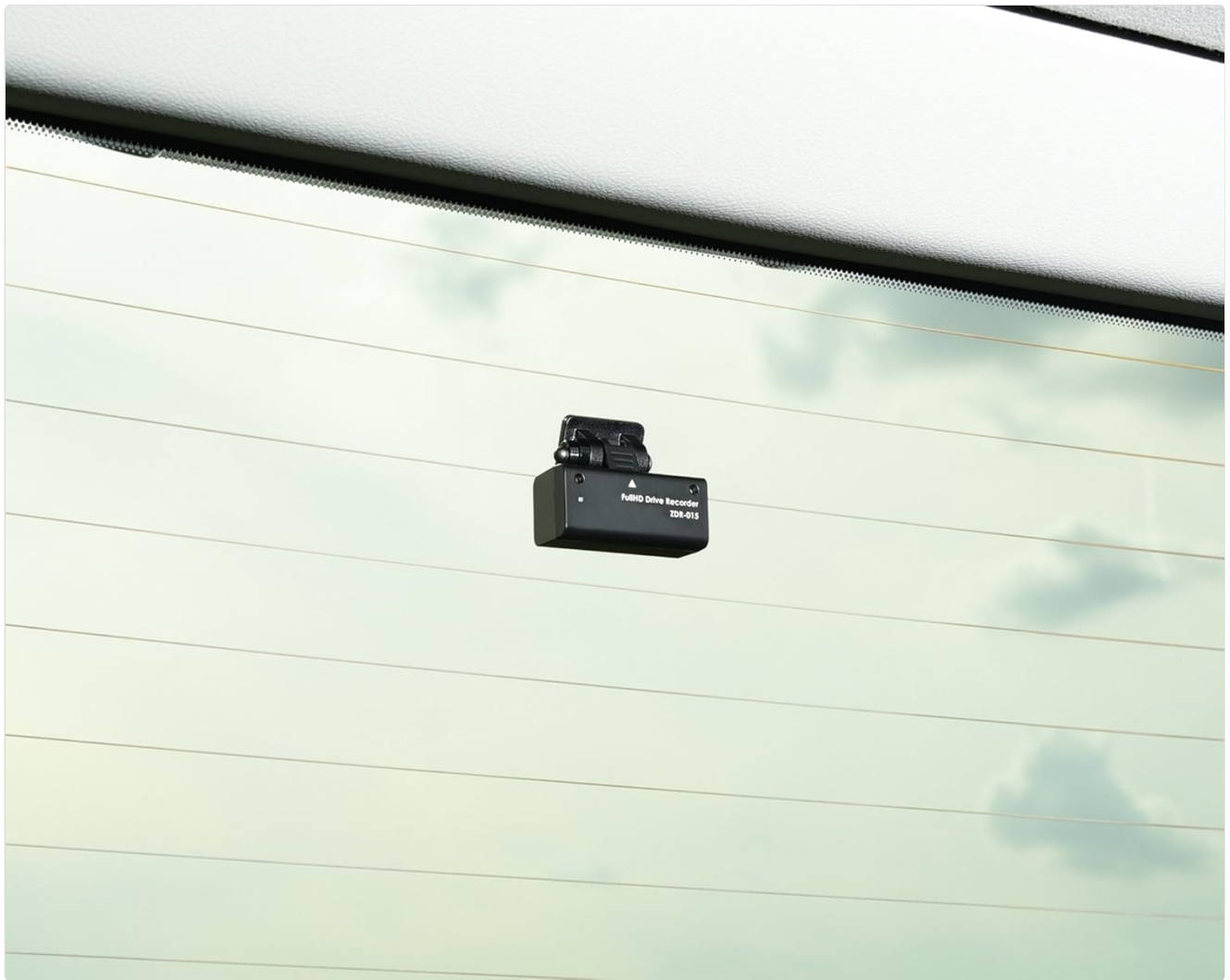
Image: Rear camera installed on the car's rear window, capturing footage from behind the vehicle.
