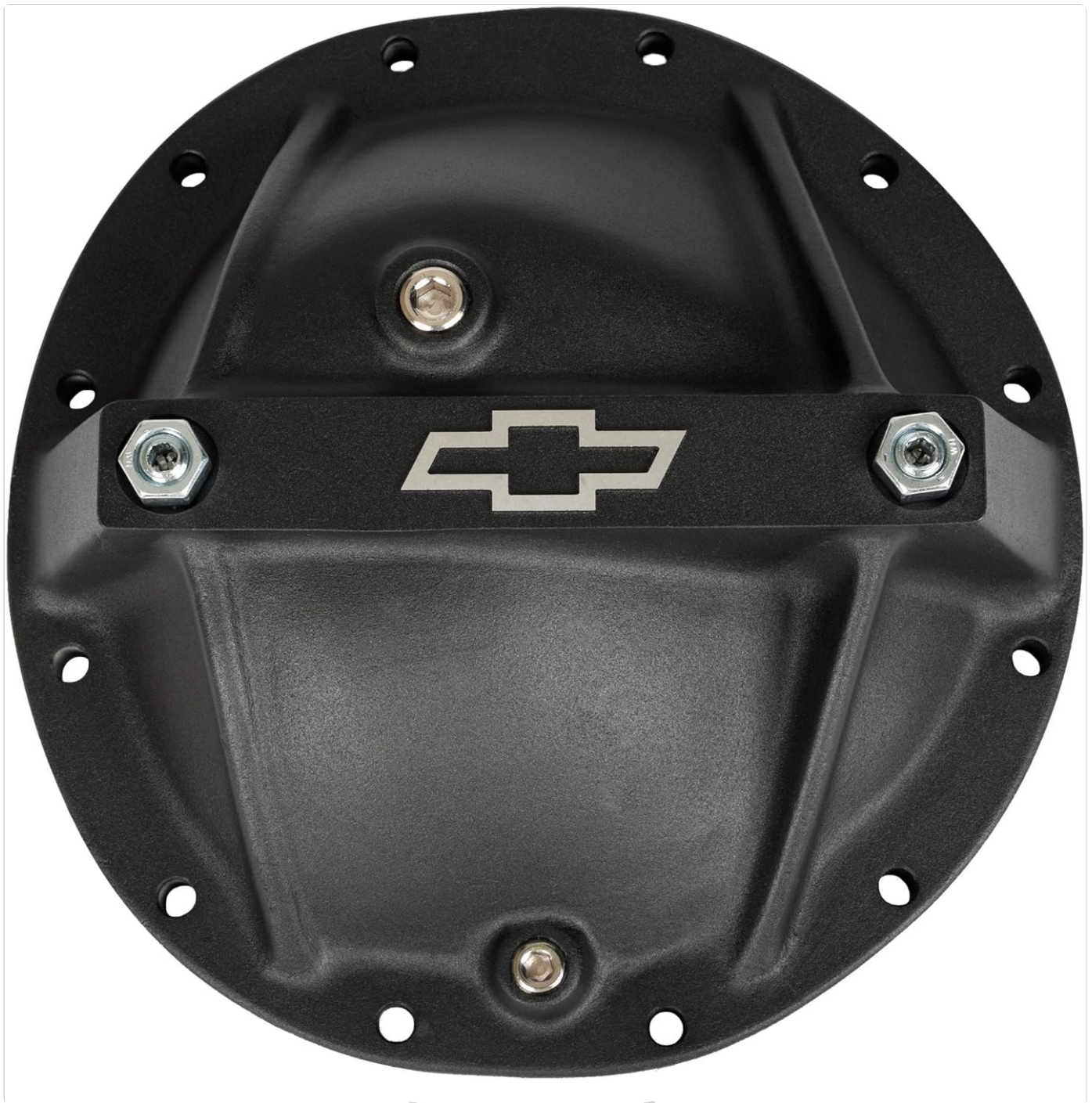
Figure 1: Proform 141-697 Reinforced Differential Cover. This image shows the black crinkle powder-coated aluminum differential cover with the Chevrolet bowtie logo, main cap bolts, and magnetic drain plug visible. The cover features a reinforced design for enhanced durability.
