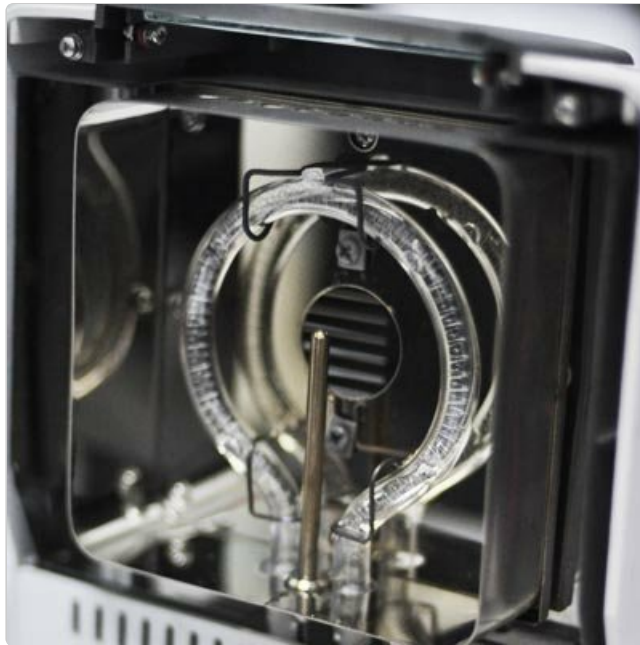
Figure 2: Detailed view of the halogen heating element, responsible for drying the sample. Ensure this area is kept clean and free from obstructions.
