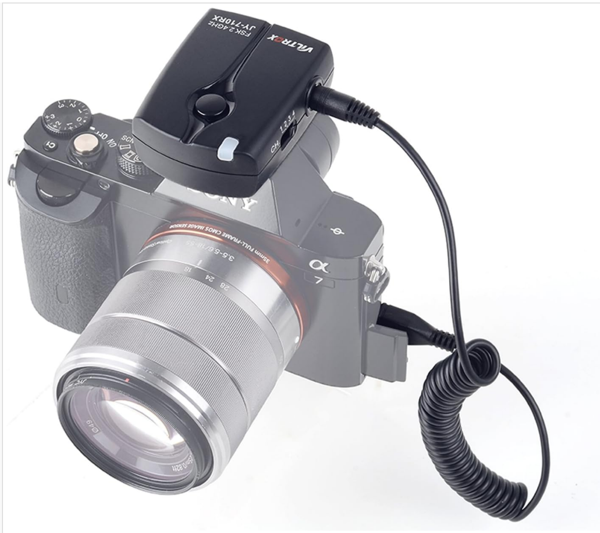
Image: The VILTROX JY-710-S2 receiver securely mounted on a Sony camera's hot shoe and connected via the S2 cable.
