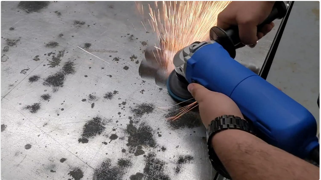
Figure 3: Zirconia flap wheel in use for grinding metal, producing sparks.
