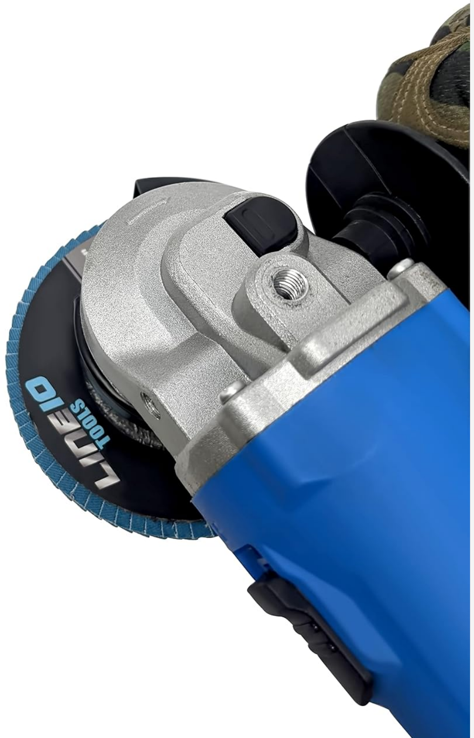
Figure 4: Aluminum Oxide flap wheel attached to an angle grinder, ready for use.
