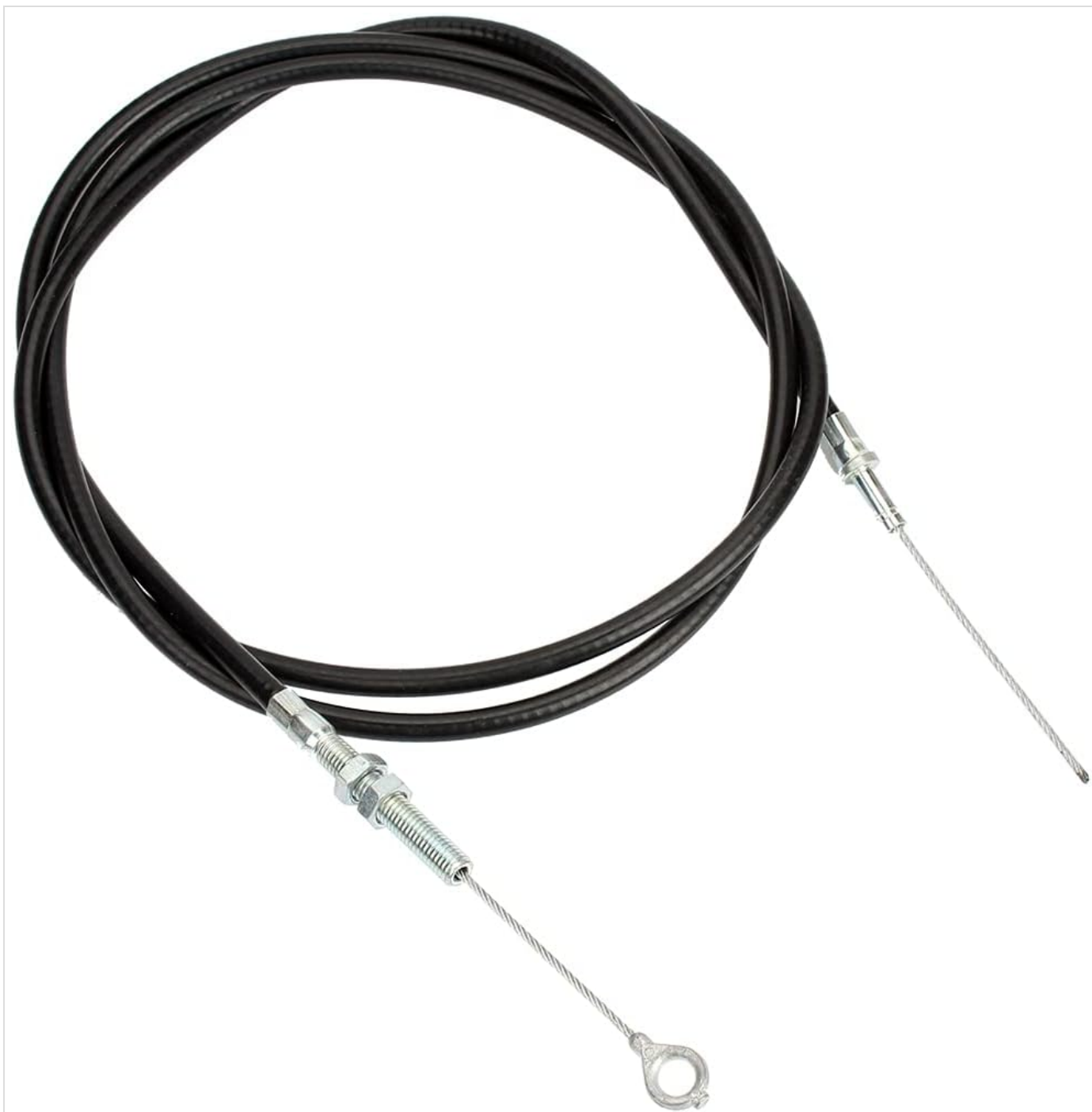
Figure 3.1: The DKIIGAME throttle cable, coiled for packaging, showing both ends.
