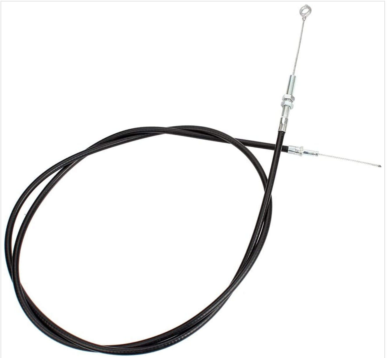
Figure 5.2: The throttle cable showing both connection ends, one with an eyelet and the other with a crimped wire end.
