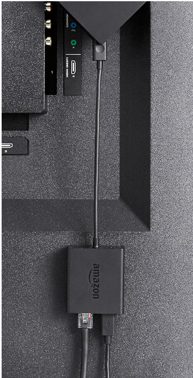
Figure 4.2: A complete setup showing the Amazon Ethernet Adapter connected to a Fire TV device, which is then plugged into an HDMI port on a television, with the Ethernet cable connected to the adapter.
