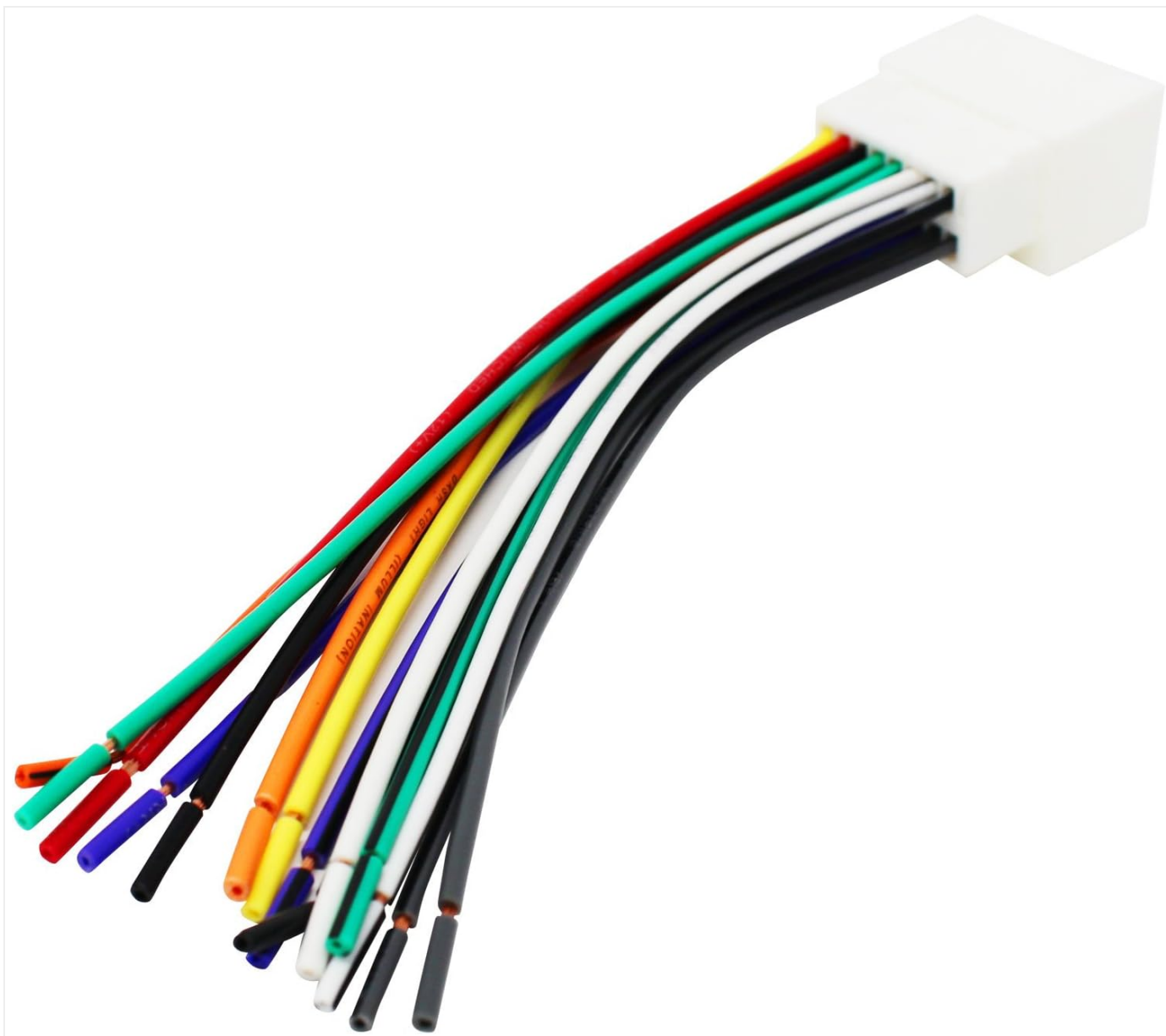
Figure 3: The opposite end of the wiring harness, displaying the individual color-coded wires with pre-stripped ends, ready for connection to the aftermarket stereo's wiring.
