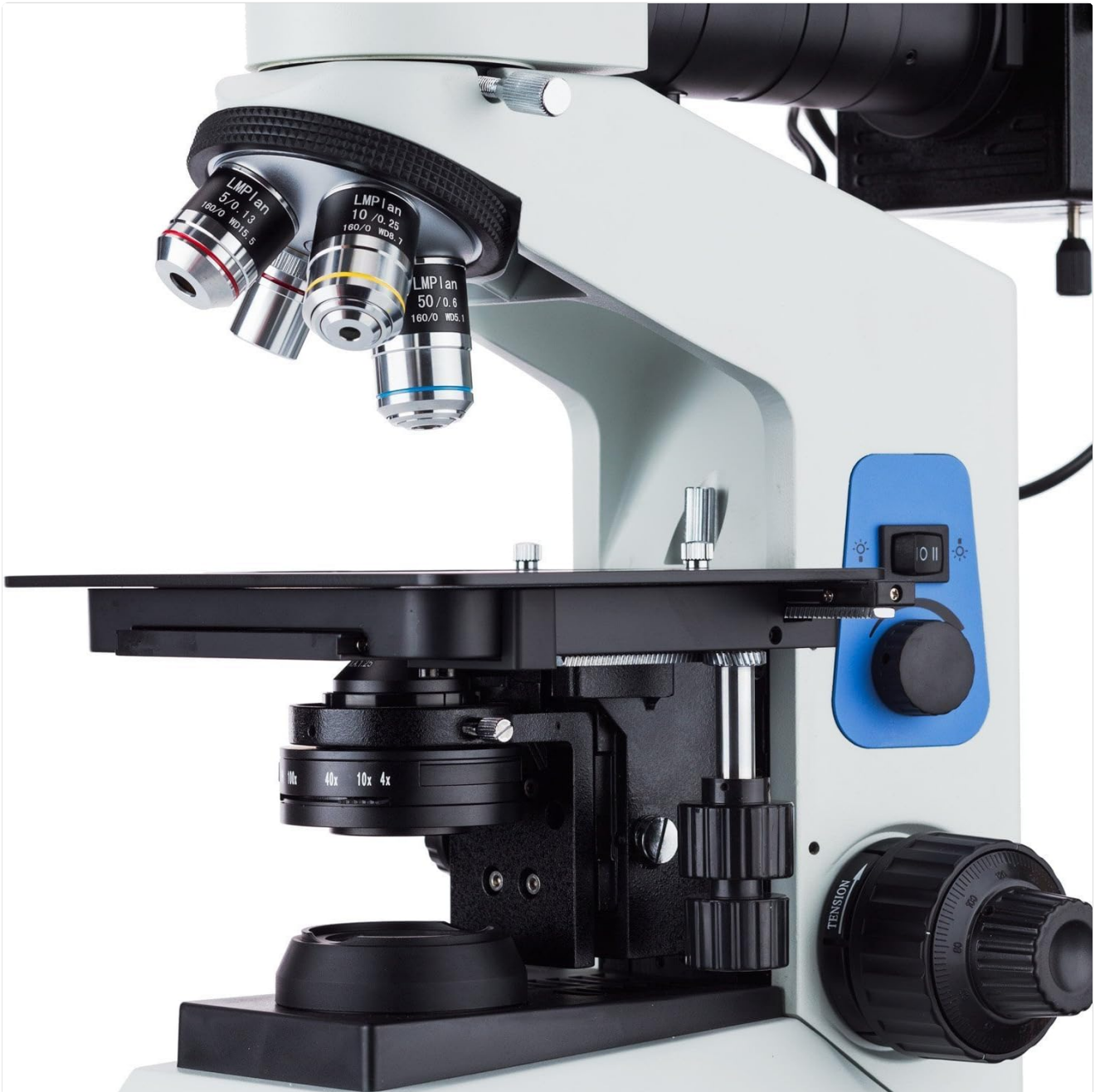
Figure 2: Close-up of the microscope stage, objective turret, and control knobs. This view highlights the mechanical stage, the objectives mounted on the revolving nosepiece, and the coarse/fine focus knobs.
