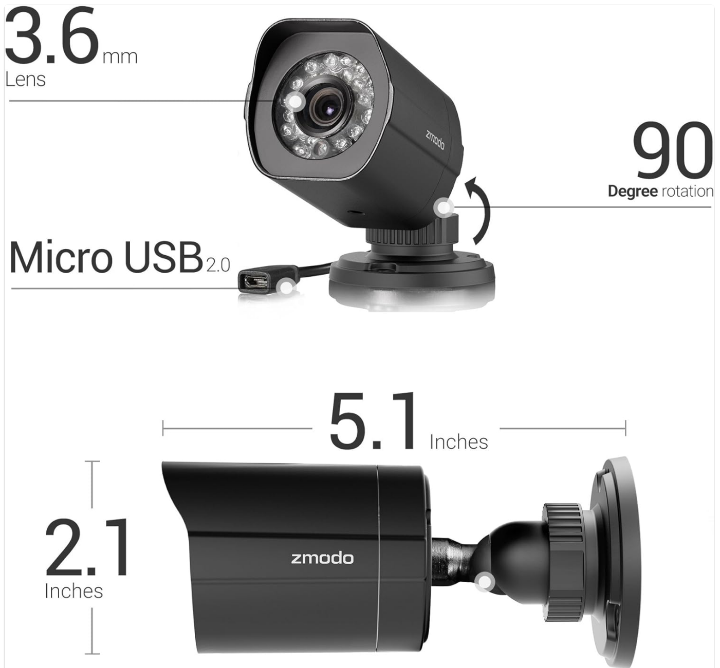
Image: Detailed view of a Zmodo camera, highlighting its 3.6mm lens, 90-degree rotation capability, micro USB 2.0 port, and overall dimensions (2.1 inches height, 5.1 inches length).
