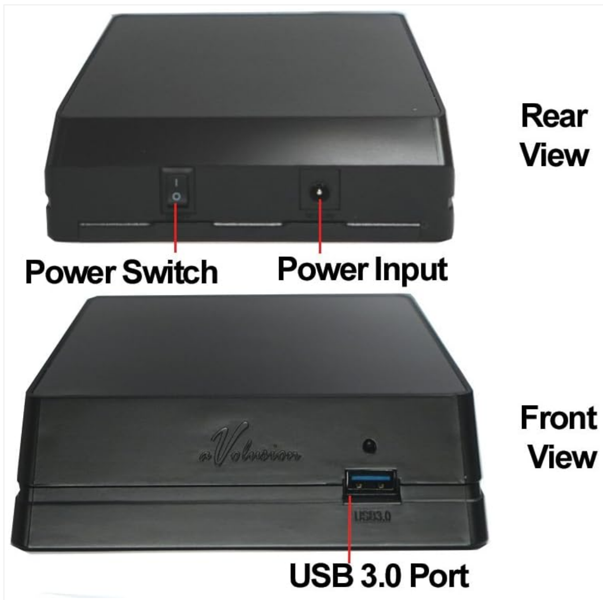
Image: Front view showing the USB 3.0 Port and rear view showing the Power Switch and Power Input.
