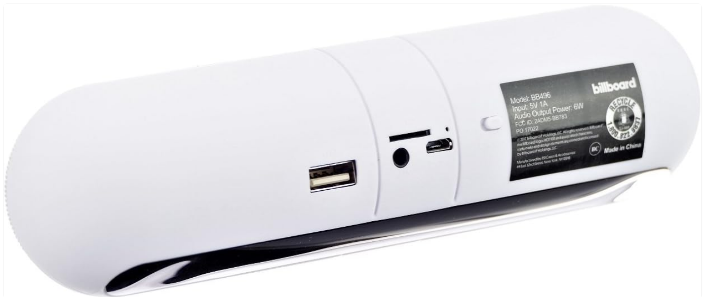
Figure 3: Rear view of the Billboard BB496 speaker, highlighting the various input ports: USB, Micro SD card slot, AUX input, and Micro USB charging port.
