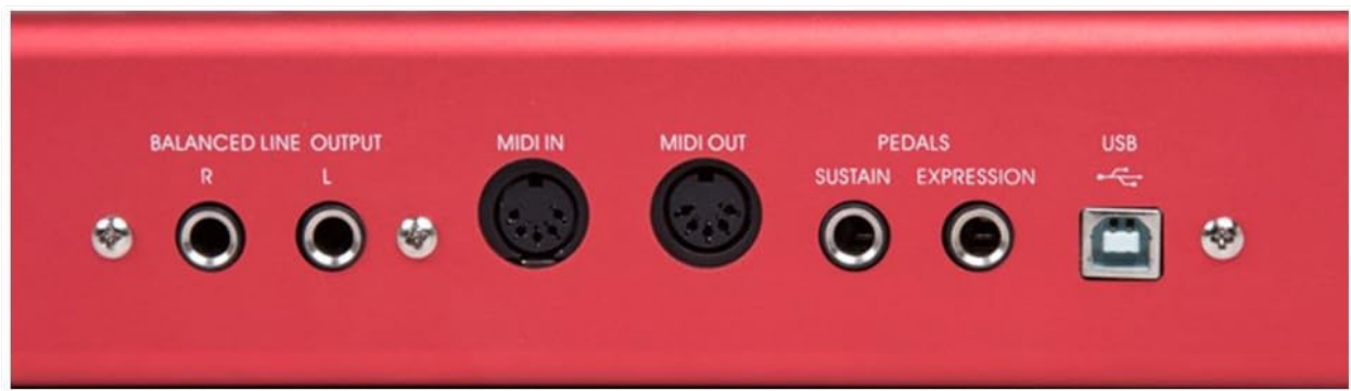
Figure 4.3: Rear panel of the Midiplus X8 Pro, showing the various input and output ports. From left to right: Balanced Line Output (R, L), MIDI In, MIDI Out, Pedals (Sustain, Expression), and USB port.
