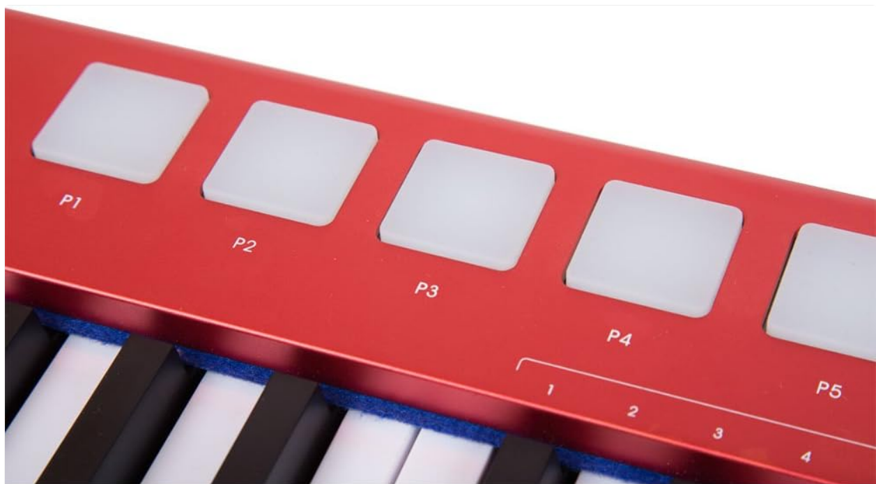
Figure 4.5: Close-up view of the 8 velocity-sensitive drum pads on the Midiplus X8 Pro. These pads are illuminated and can be used for triggering samples, drums, or other MIDI events.
