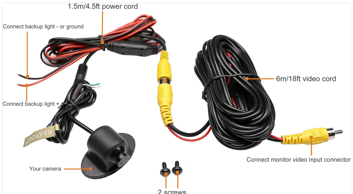
Figure 2.3: Wiring Diagram. This diagram illustrates how to connect the camera's power cord to the vehicle's 12V power source (e.g., backup light) and the video cord to the monitor's RCA input. It also shows the included screws.
