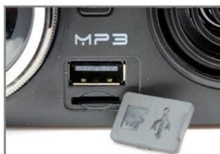
Figure 4.1: Various input ports including USB, SD card slot, and AUX interface.
