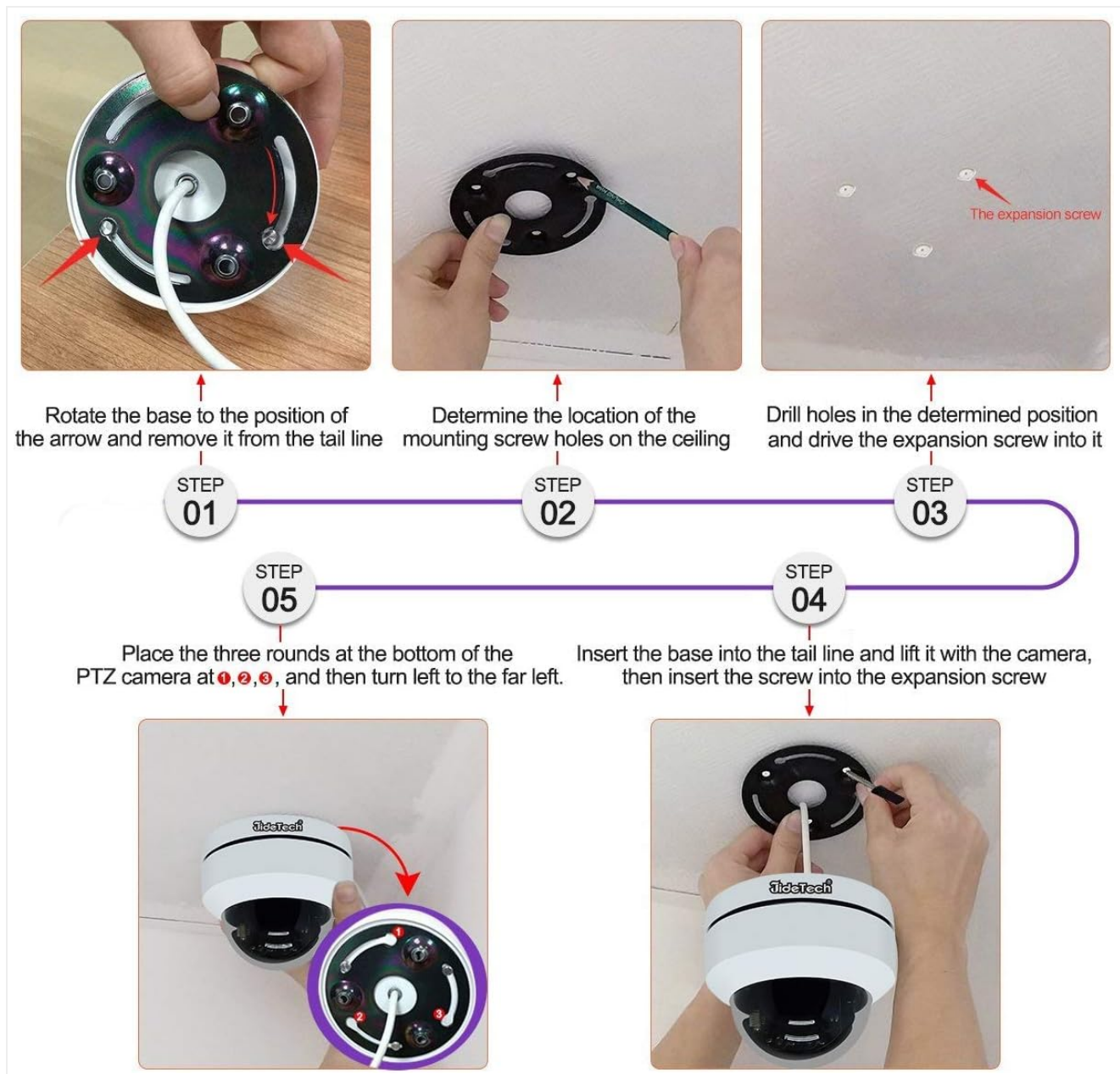
Figure 4.1: Physical installation steps for the dome camera.
