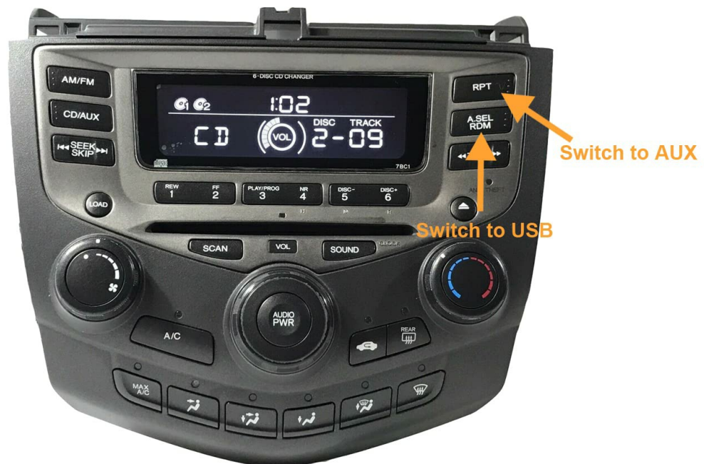
Image 6: Car radio controls for switching between audio sources.
