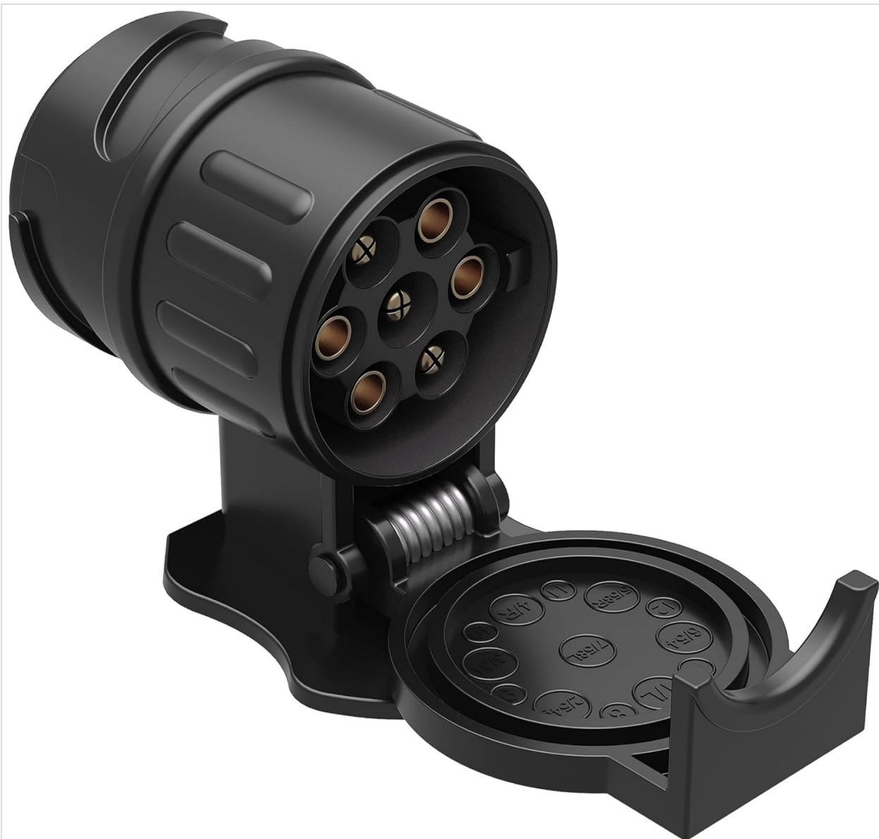
Figure 2.1: WilTec 13 to 7 Pin Trailer Adapter, front view with 7-pin socket visible. This image shows the WilTec 13 to 7 Pin Trailer Adapter. The adapter features a robust black plastic housing with a hinged cover for the 7-pin socket, designed to connect a 7-pin trailer to a 13-pin vehicle socket.
