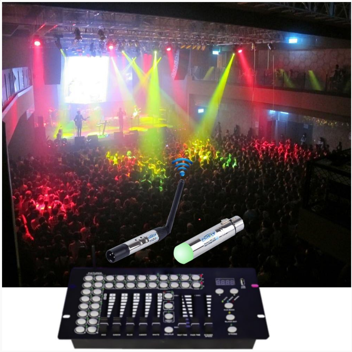
Figure 5.1: An example of the CHINLY DMX wireless system integrated into a stage lighting setup, showing the transmitter connected to a DMX console and receivers connected to lights.
