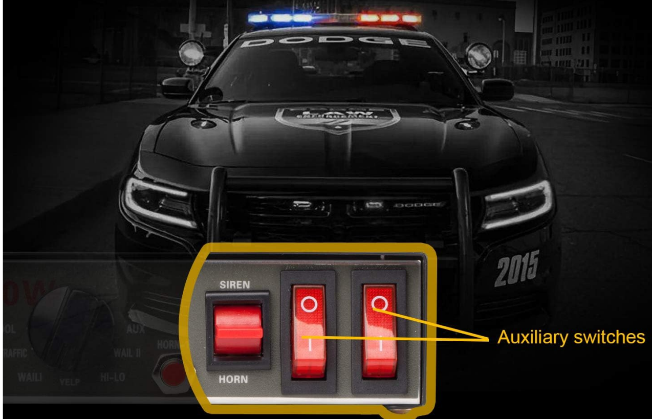
Image 6.1: The two auxiliary switches on the control box for external light control.
