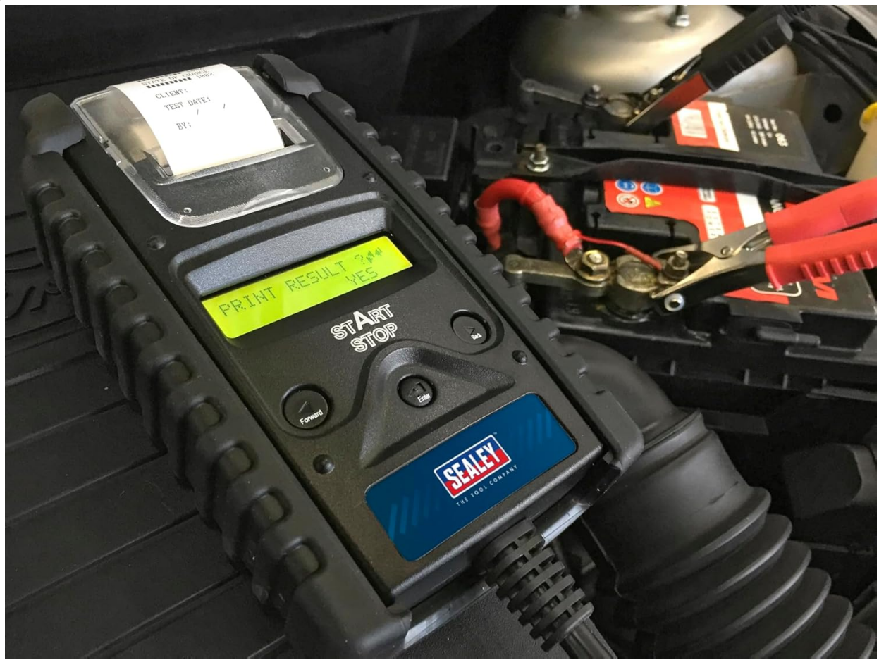
Figure 6.1: The Sealey BT2014 tester actively performing a test on a vehicle battery, with the display showing a prompt to print results.
