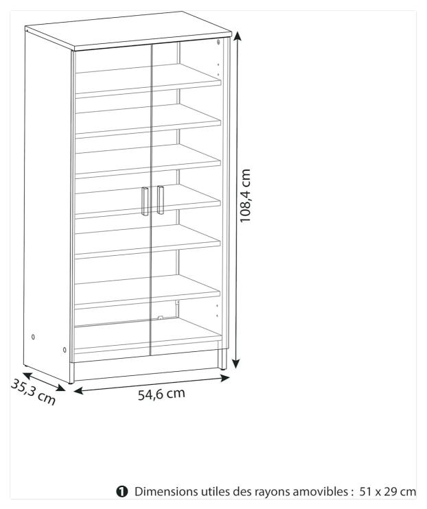
Figure 3: Cabinet dimensions and useful shelf dimensions for assembly planning.
