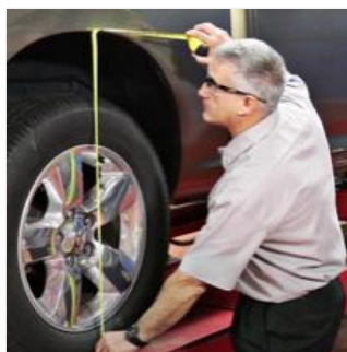
Image: A technician uses a tape measure to record the vehicle's ride height from the wheel arch to the center of the wheel, a crucial step before and after strut replacement.
