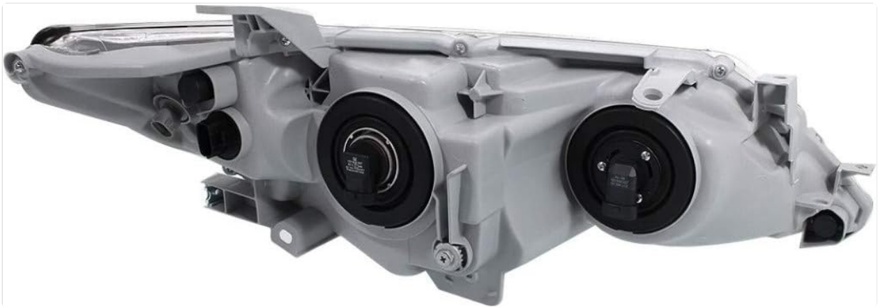
Figure 2: Rear view of the headlight assembly, illustrating bulb sockets and mounting points.
