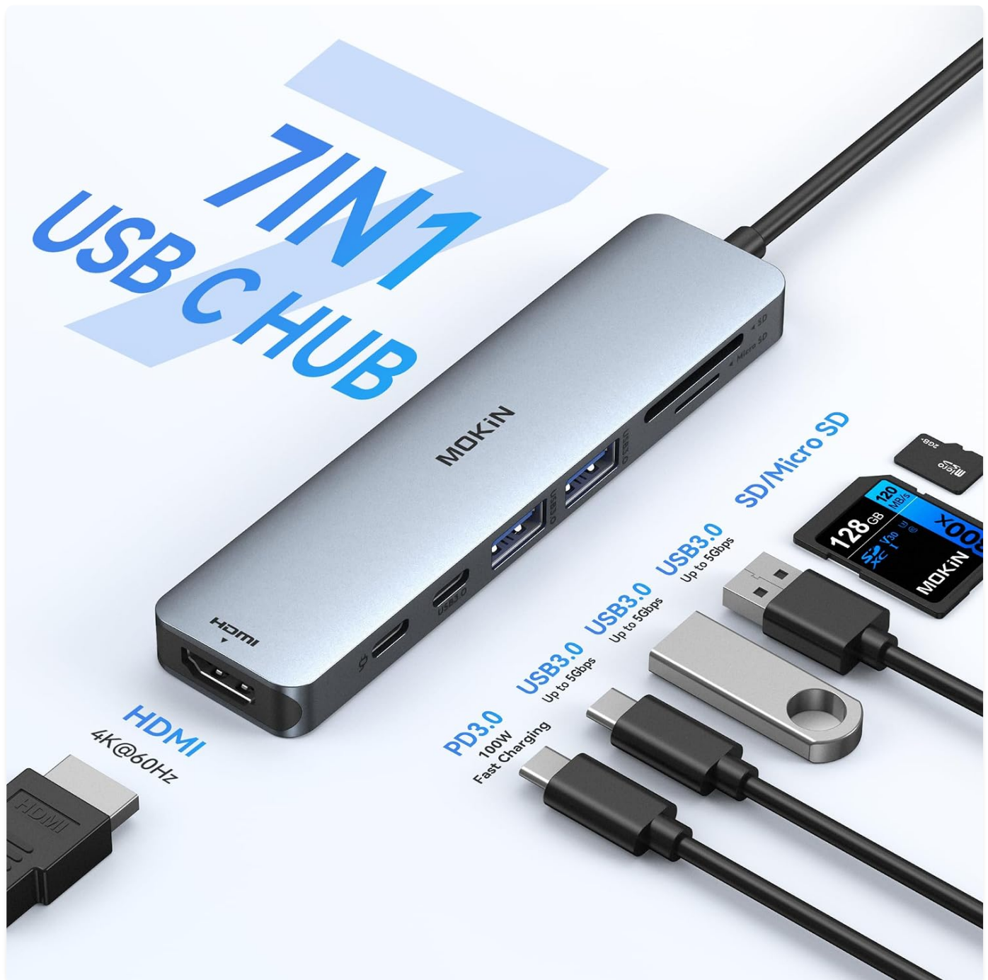
Figure 2.2: Detailed view of the MOKiN 7-in-1 USB C Hub ports.
