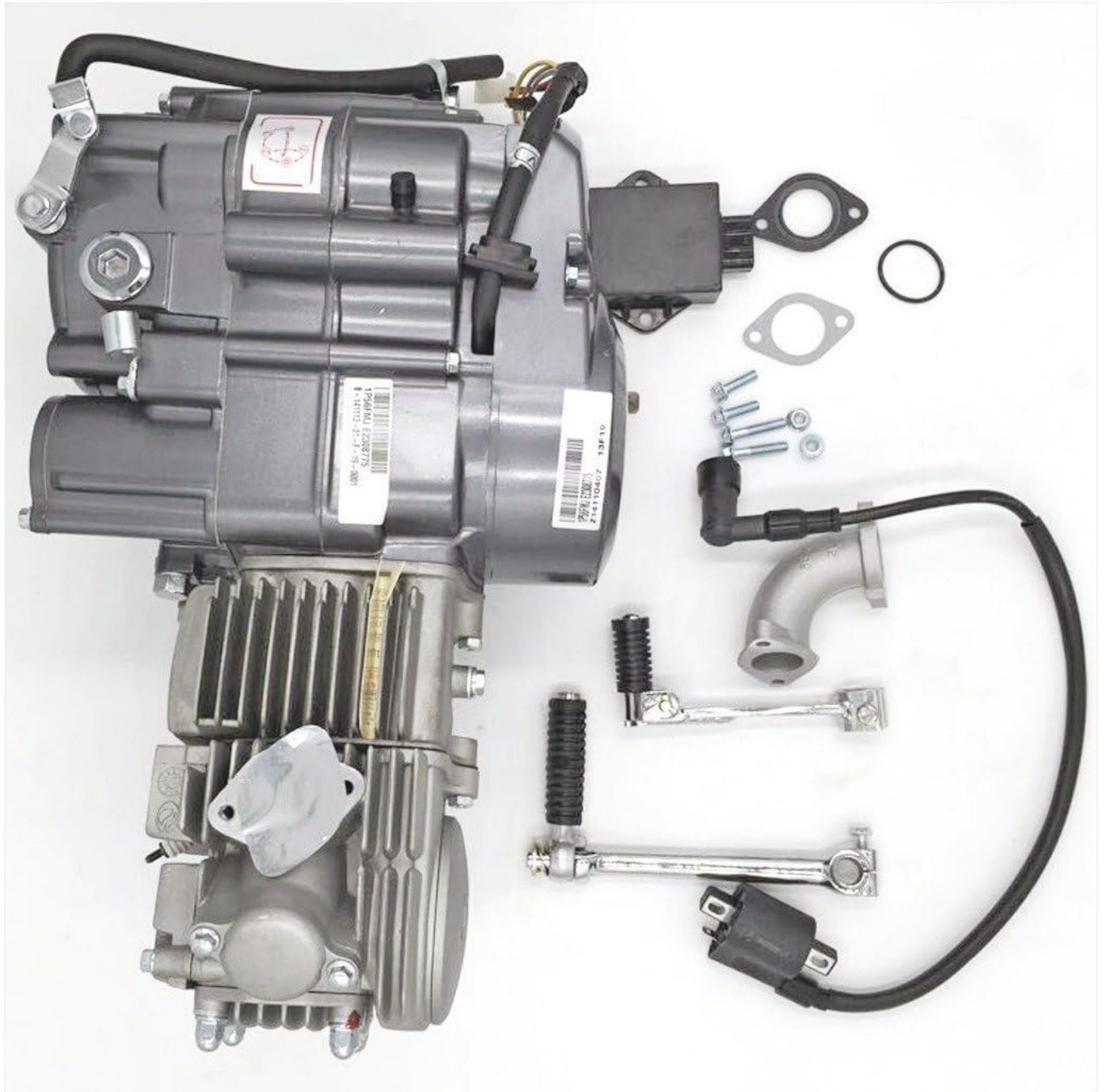
Image: Side view of the ZXTDR Lifan 150cc engine, highlighting various components and mounting points.
