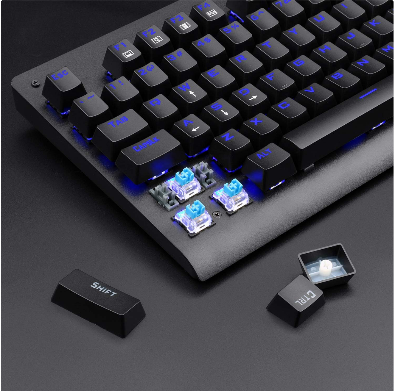
Image: Close-up view of the mechanical blue switches on the EagleTec KG040 keyboard, with some keycaps removed to show the switch mechanism.
