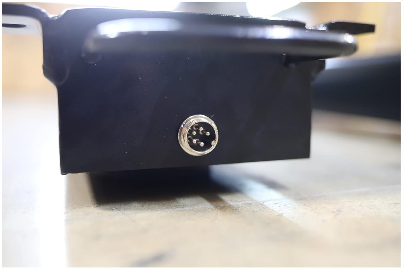
Image 4.2: A close-up view of the circular connector port on the weigh bar, where the signal cable is attached.
