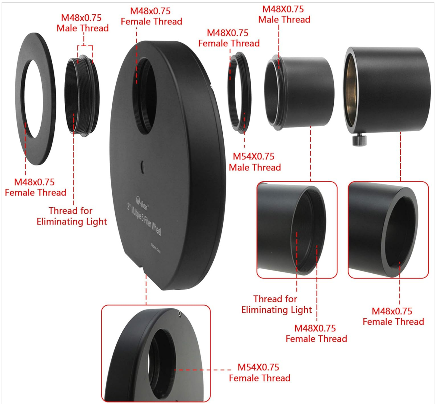
Figure 2: Detailed view illustrating the various thread types and adapters for the filter wheel, including M48x0.75 male/female threads, M54x0.75 male/female threads, and threads for eliminating light.
