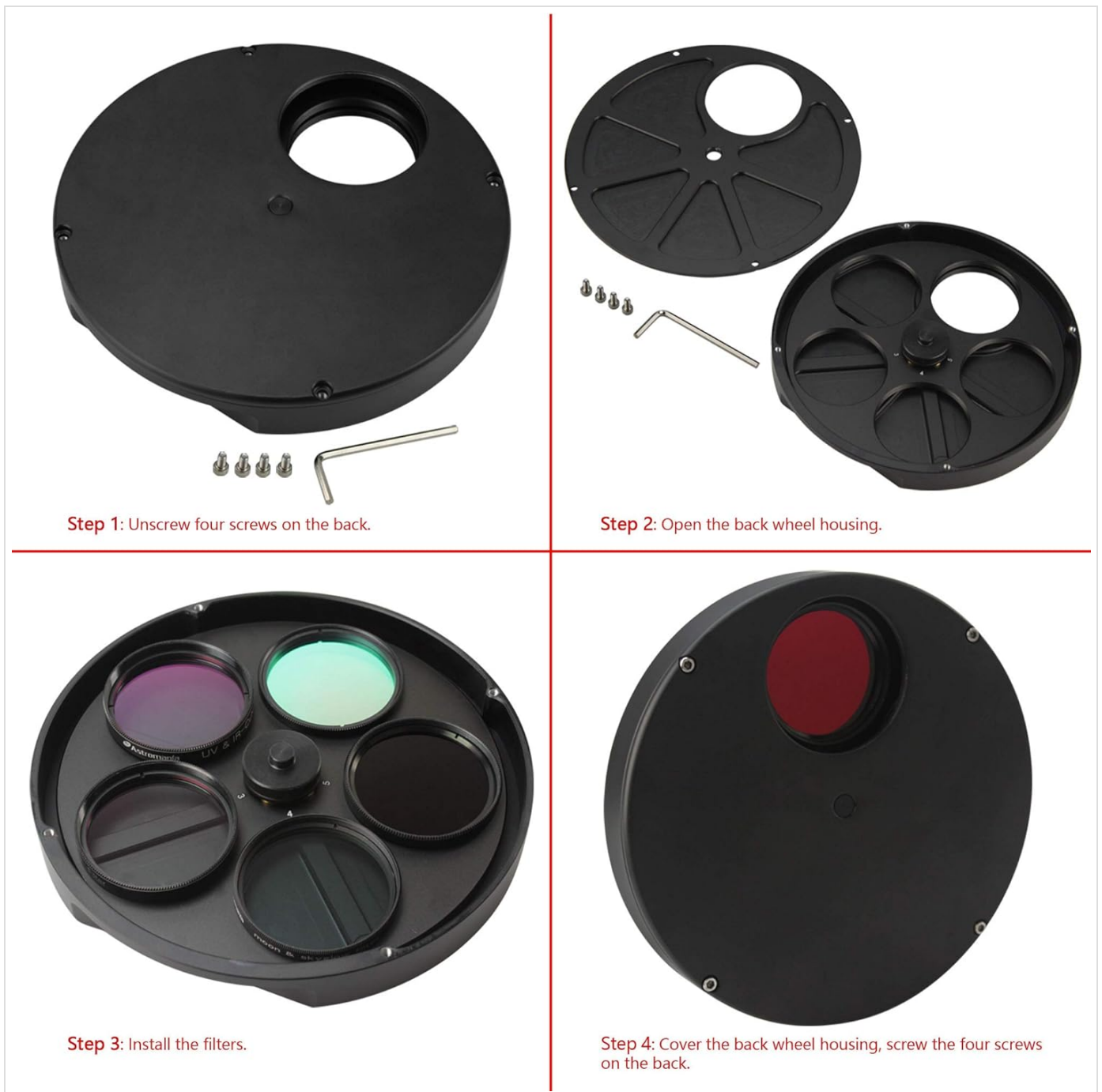
Figure 3: Step-by-step guide for installing filters: 1) Unscrew back, 2) Open housing, 3) Install filters, 4) Cover and screw back.
