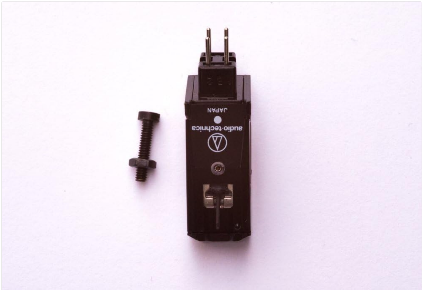
Figure 2: Top view of the AT Cartridge, showing the connection pins and the fixing bolt.
