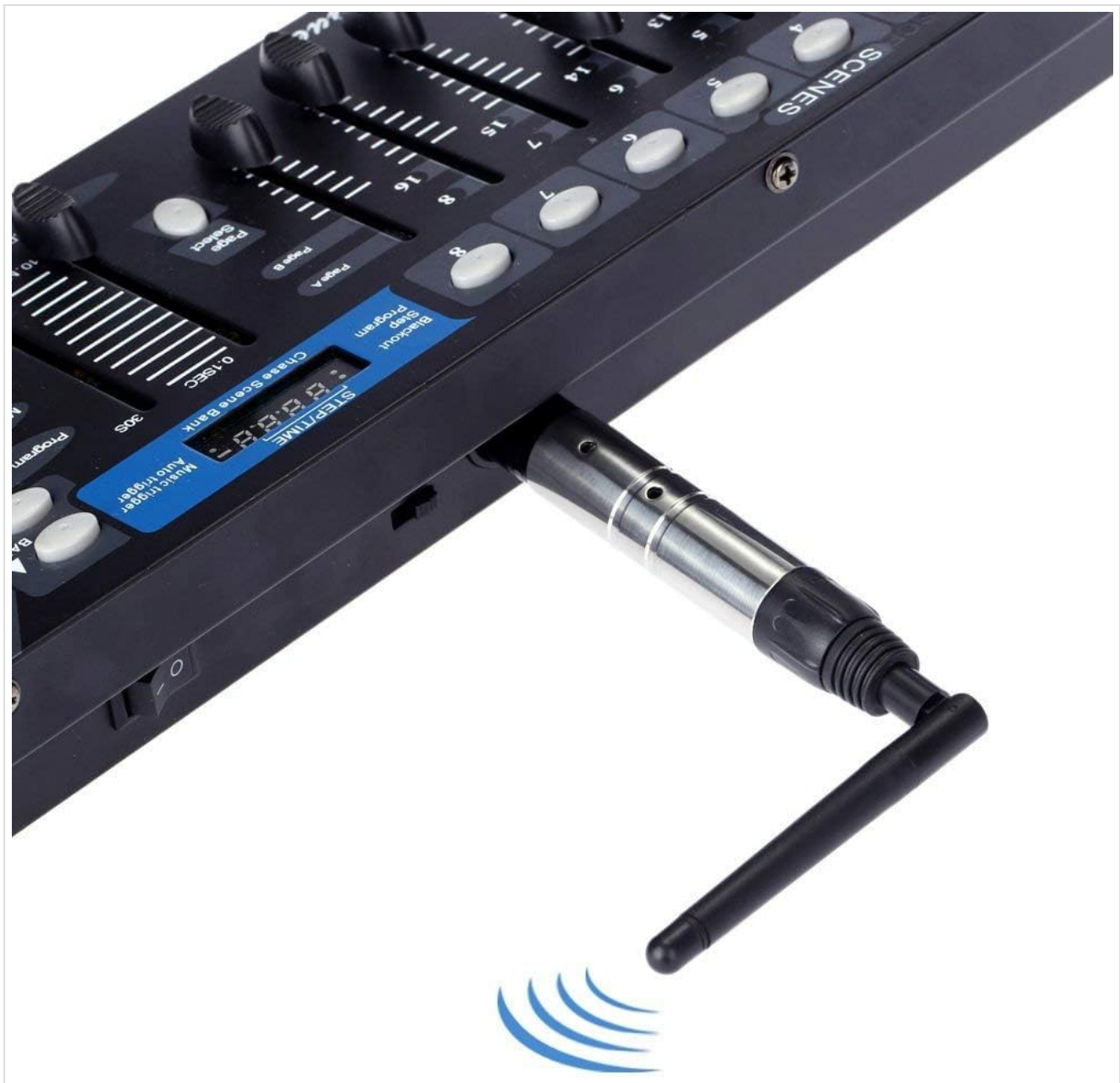
Image 5.1: The DMX transmitter connected to a lighting control console.
