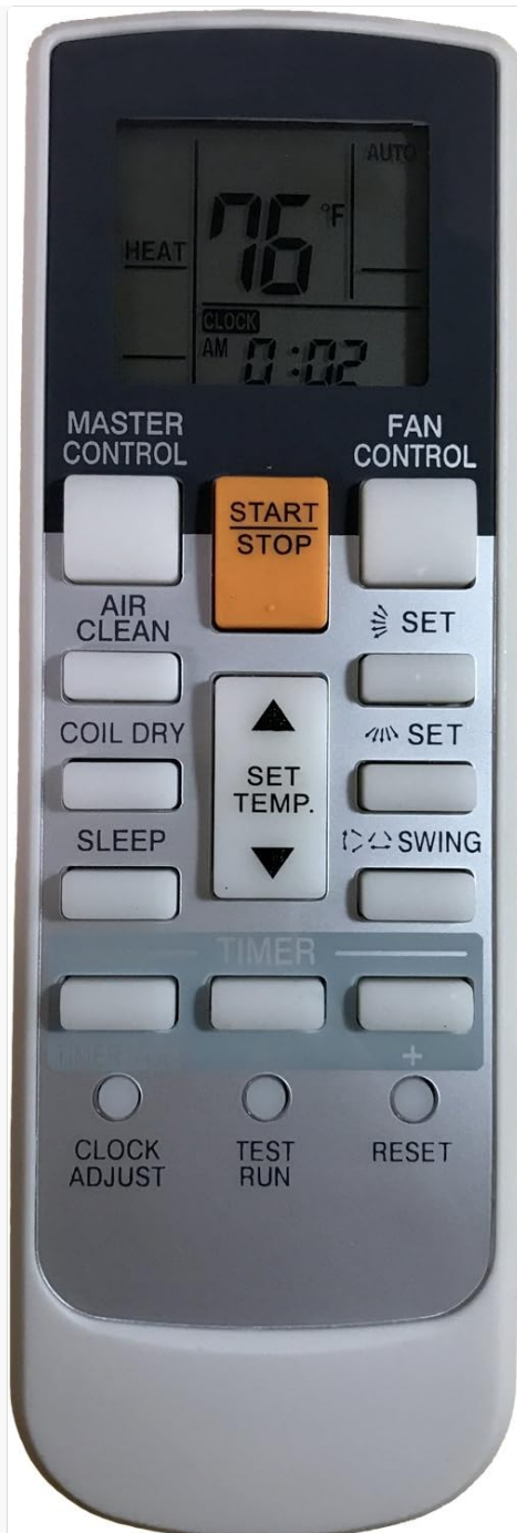
This image shows the front of the remote control, with a magnified view of the LCD screen displaying '76 °F' and 'HEAT' mode, confirming Fahrenheit display.
