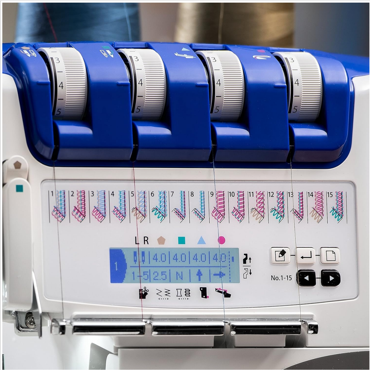
Figure 5: Close-up of the LCD display and tension adjustment dials on the JUKI MO-2000QVP.
