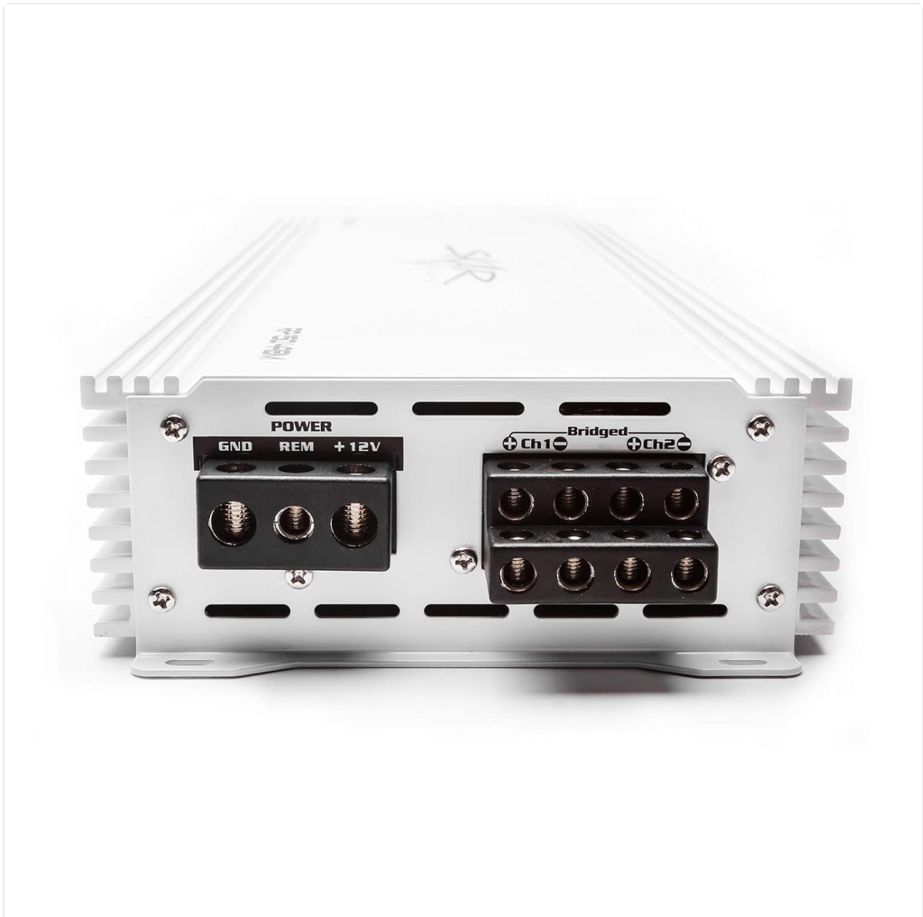
Figure 2: Power and speaker terminal side of the amplifier. Note the two sets of speaker terminals for convenience with thicker wires, though it functions as a single mono block output.
