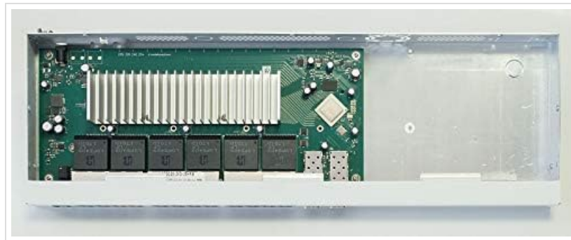
Figure 2: Internal view of the MikroTik CRS326-24G-2S+RM switch, revealing the circuit board, heatsink, and SFP+ module slots. This view is for informational purposes and the device should not be opened by unauthorized personnel.
