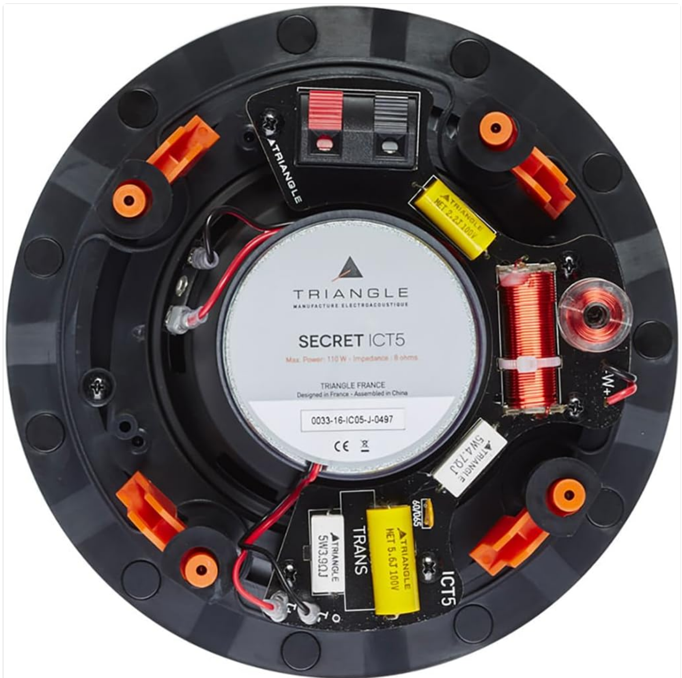
Image: The rear view of the Triangle Secret ICT5 speaker, displaying the red and black spring-loaded wiring terminals, crossover components, and the central magnet structure.
