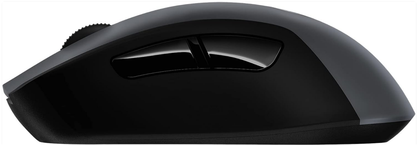
Figure 5: Side view of the Logitech G603, highlighting the two programmable thumb buttons.
