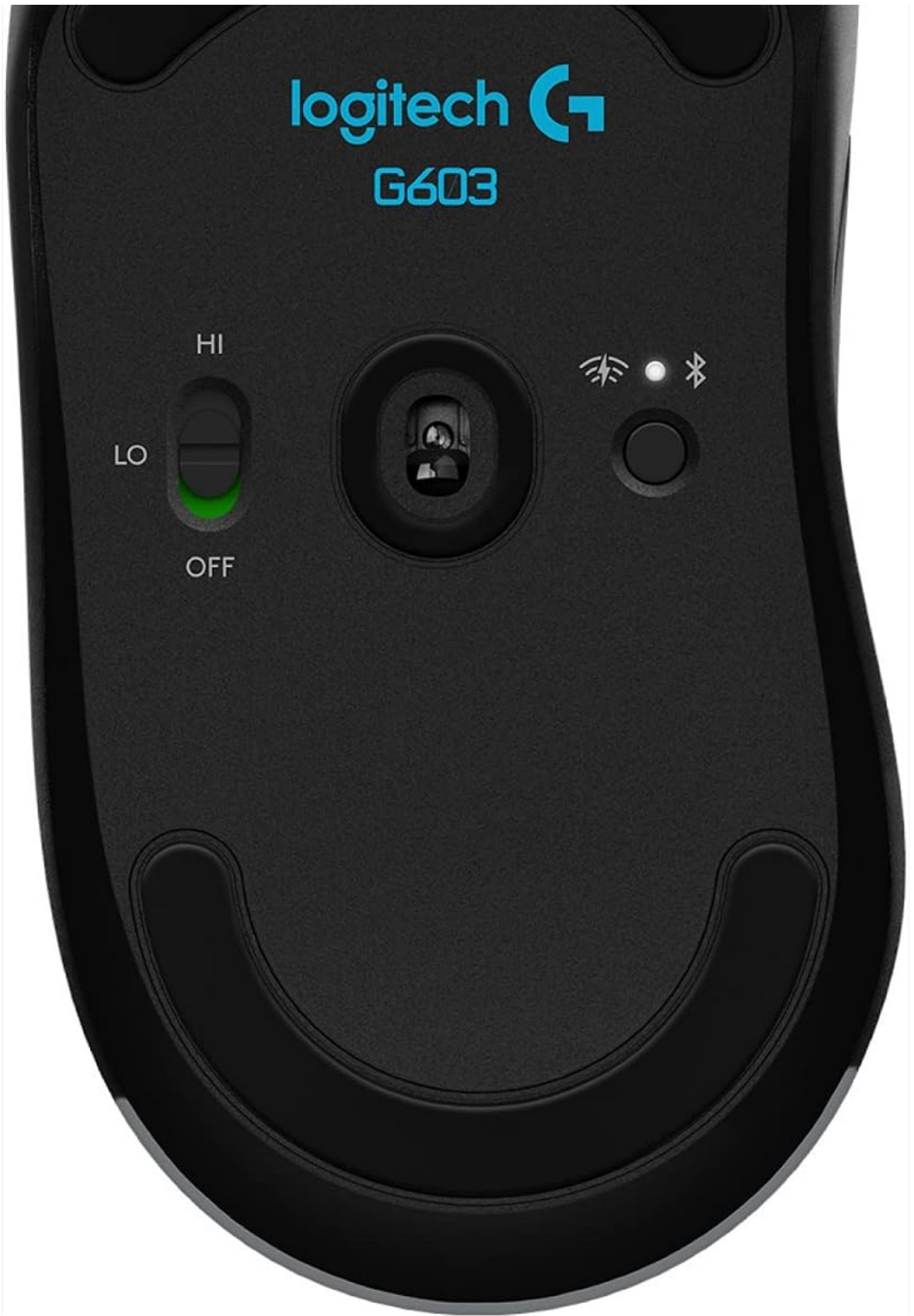
Figure 4: The bottom of the Logitech G603, showing the HI/LO power switch and the Bluetooth pairing button.
