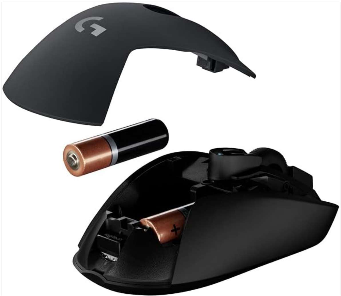
The Logitech G603 mouse with its top cover removed, revealing the two battery compartments for AA batteries.
